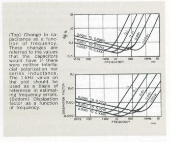
Dissipation Factor: Not greater than 0.001, 0.0005, and 0.0003 for capacitances of 100 to 1000 pF, 1100 to 2000 pF, and 2100 pF to 1.1110 µF, respectively.
